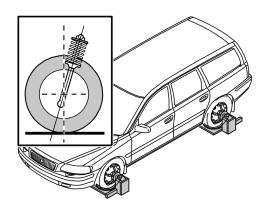
The caster angle must not vary by more than 0.25° between the left and right-hand sides.
