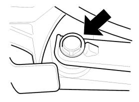
adjusted in relation to each other on the front and rear axles. This is extremely important so that the rear wheel toe angle can be adjusted in relation to the car's thrust line (geometric driving axis). The thrust line is the line created when the toe angles for the rear wheels are equally divided. See the illustration. The difference between the symmetry line of the wheels and the thrust line is called the thrust angle. The thrust angle must not deviate by more than
