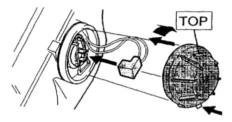
Press the connector into place on the bulb.
