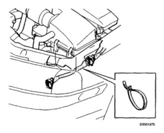
Secure the adapter cable using a tie strap around the existing cable between the fender liner and the air cleaner (ACL) housing.
