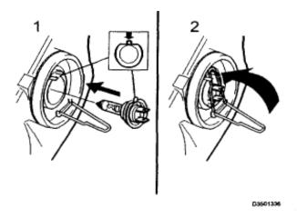
Insert the new bulb with the guide lug upwards, without touching the glass (1). The bulb will seat properly only in this position.
