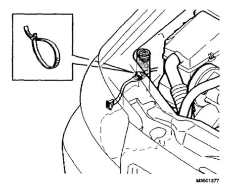
Remove the filler pipe for the windshield washer fluid. Secure the adapter cable using a tie strap around the fluid filler pipe.
