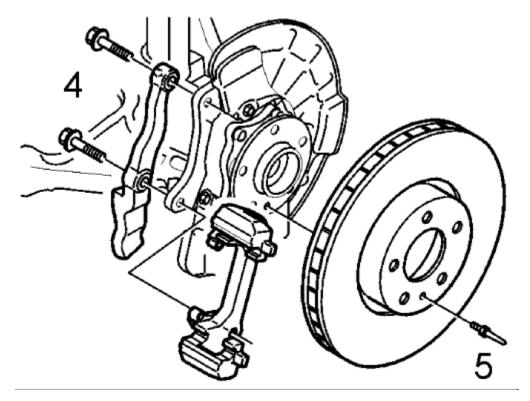
Install the locating pins in the <u>brake caliper</u> Install the wheel
