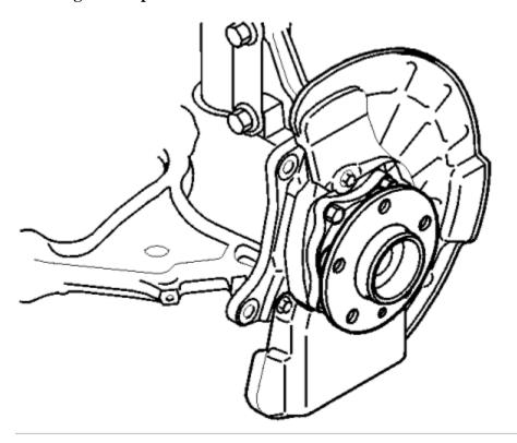
**NOTE:** Cleaning is important to prevent lateral runout at the brake disc
