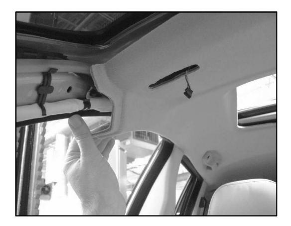
Disassemble the <u>sun visors</u> and the front interior light panel according to VADIS.
