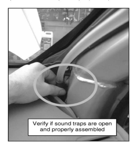
Disassemble A-pillar panels according VADIS. Pull the rubber sound traps out of the holes in the front A-pillars and verify that they are open and clear from debris or dirt.
