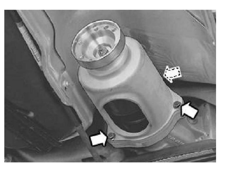
Position a drip pan under the final drive and viscous coupling.
