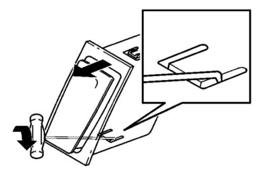
Turn the special tool clockwise. At the same time pull the cup holder out at the bottom edge.
