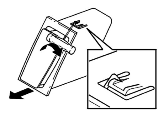
Carry out the same procedure to disconnect the hook at the top of the cup holder.
