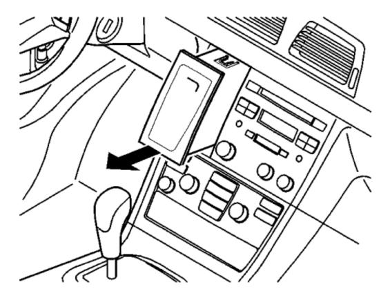
\* Pull the cup holder straight out and remove.
