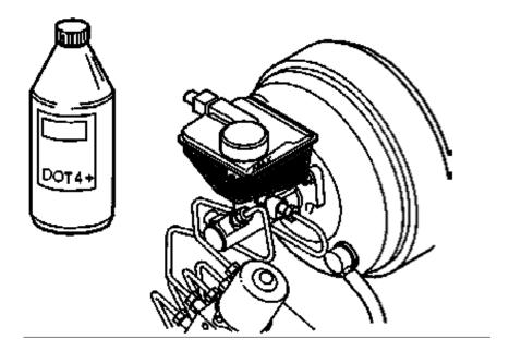
When reconditioning or replacing brake calipers bleed the relevant brake pipe as follows. The brake pedal must be depressed throughout the operation. This is so that the brake system is not drained of brake fluid.
