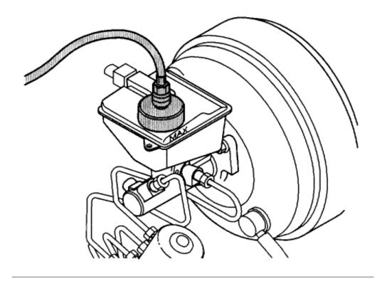
Close the cock on the pressure line. Open a nipple and close it again. Checking for air in the brake system and for brake fluid leakage See Brake pipe master cylinder / ABS unit, replacing
