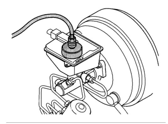
Connect bleeding unit to brake fluid reservoir. Follow manufacturer's instructions for connecting and using bleeding unit.
