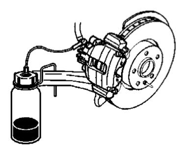
Remove the protective cap from the bleed nipple. Connect the hose from the collection bottle. Open the bleed nipple. Close it when there are no more air bubbles in the fluid coming out of the hose.
