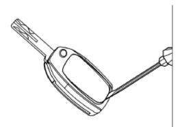
Remove the screw and separate the unit.
