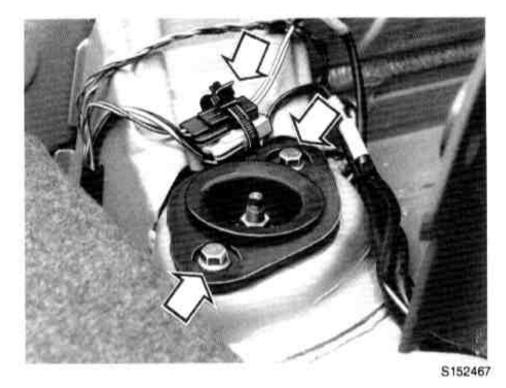
Raise the rear suspension so that the wheels are clear of the around. Remove the two upper shock absorber mounting screws.
