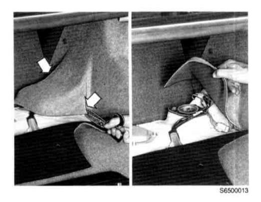
Cut side panel vents in the front and rear edges as illustrated. Turn up the panel cover that covers the shock absorber mounting.
