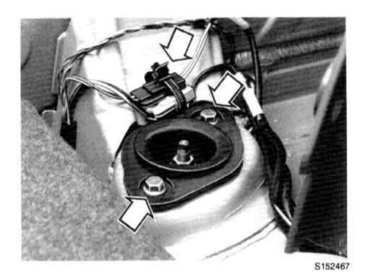
Tighten mounting screws a few turns.
