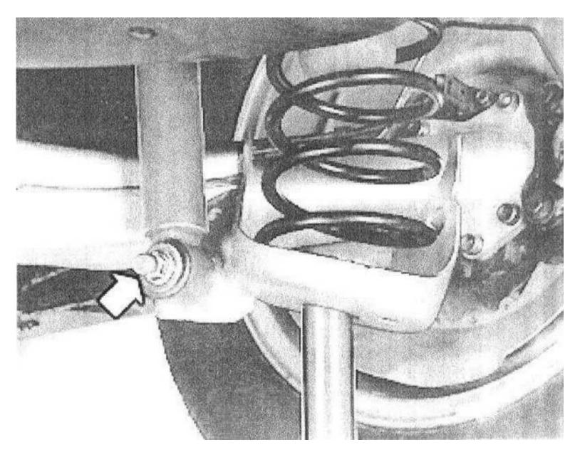
Locate the spring end in the trailing arm stamped section and locate the mounting washer guide pin in the hole on the trailing aim. Install a new nut on the mounting washer. Tighten to 40 Nm (29.5 ft. lbs.).
