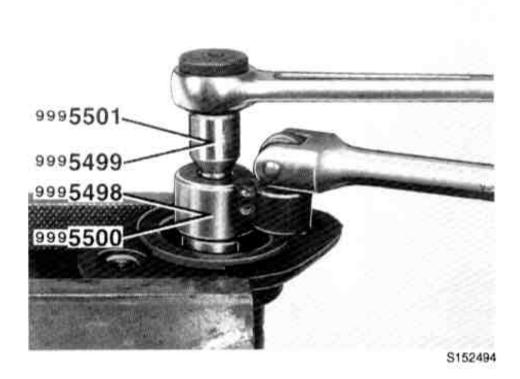
Check the mounting bushing for wear and damage. Replace if necessary. Use socket 999 5455 and wrench 999 5499 for standard shock absorbers. For Nivomat shock absorbers use socket 999 5500 and wrench 999 5501.
