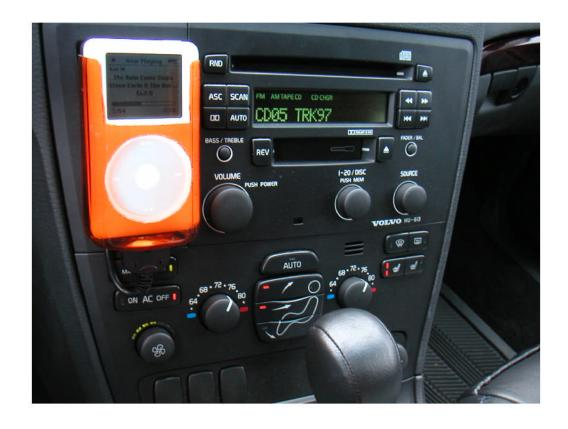
**14.** This is the finished install. As you can see, the Head unit recognizes the iPod as a CD Changer. I set both DIP switches on the PA11-VOL to off, so I can use the 1/8" AUX wire (which is coiled up behind the cradle) and use the iPod in Direct mode. The PA11-VOL makes for a much cleaner install while providing much better sound quality than a cassette adapter or an FM modulator
