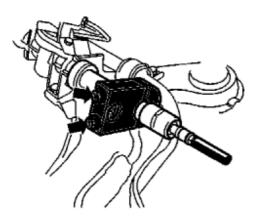
Remove the steering arm from the wheel <u>spindle</u>. Slacken off the lock nut.
