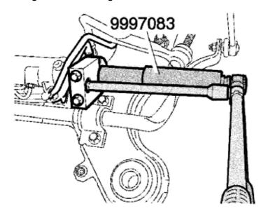
Use tool 999 7083 to remove the steering arm. Ensure that the connecting rods used are the same length. Remove the steering arm from the <u>steering gear</u>.
