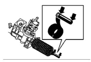
Check that the boot is undamaged.
