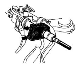
Clean the surfaces on the steering rack and the tool thoroughly. Install counterhold 999 7020.
