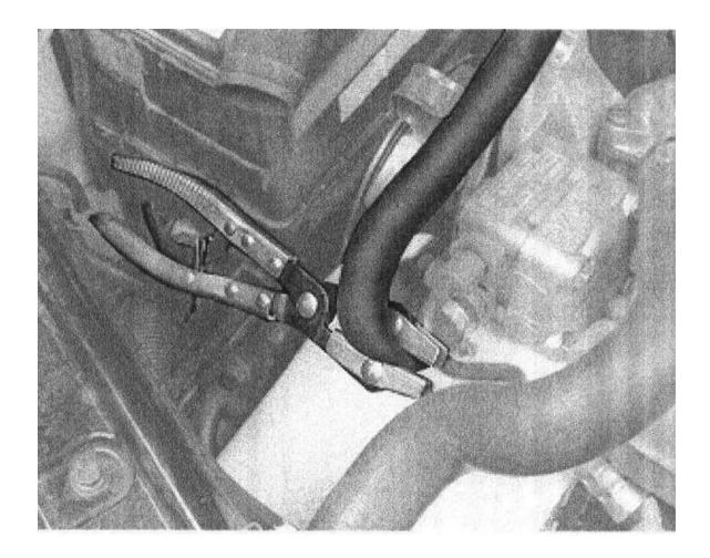
• Install lock grip pliers on the hose from the fluid reservoir as close to the power steering pump as possible.
