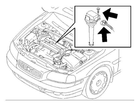
Install the cover over the ignition coil.
