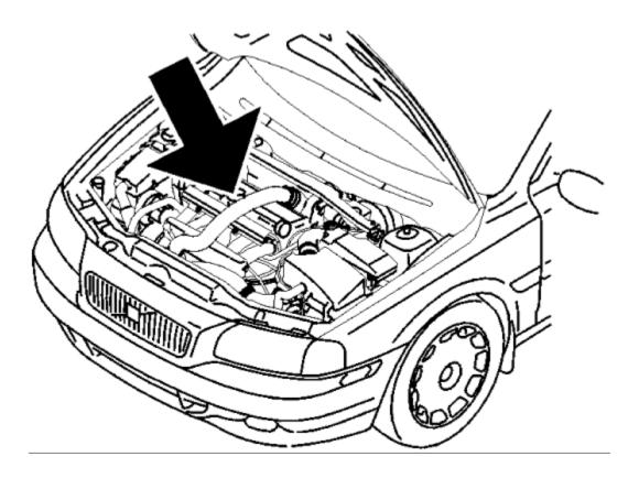
• the charge air pipe over the engine. Seal the openings
