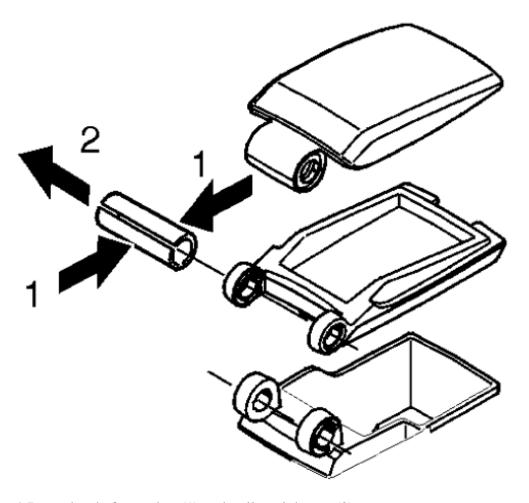
\* Press the shaft together (1) and pull straight out (2).
