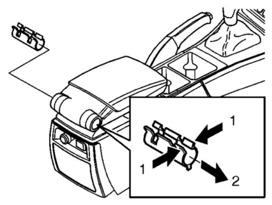
Remove the catch by pressing it together (1) and pulling it straight out (2).
