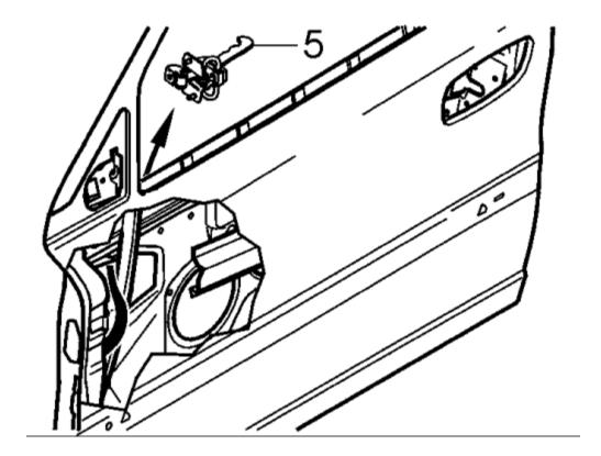
Twist the door stop carefully to remove it through the opening.
