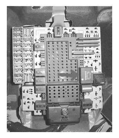
Removing the original relay
