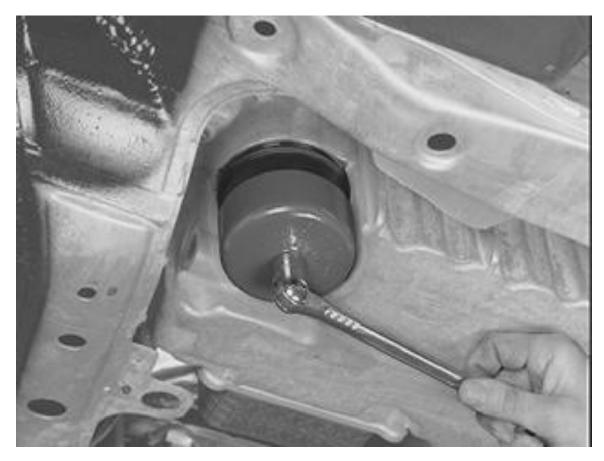
Position the container under the oil filter. Remove the oil filter housing. Use tool: 999 5679. Reinstall the oil plug again. Tighten. Always use a new sealing washer.
