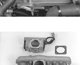
Allow the crankcase ventilation hose to run through the intake manifold without disconnecting it from the flame trap.
