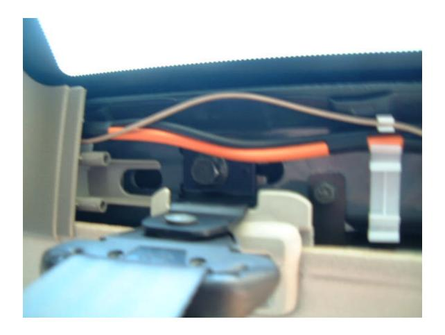
Now in the picture above you need a 14 or 15mm to undo the nut. Be very careful not to drop it as it comes out as it always rolls off somewhere diffilcut to find! After it is out the belt will still remain up as there is a small catch you just need to move up and sideways for the belts to drop to the floor. Thats it done, you are now ready to put in the steel guard.
