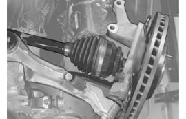
Use new screws and lock nuts for the wheel spindle and spring strut. Tighten to light contact.
