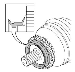
Installing the drive shaft
