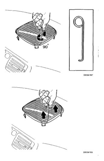
The method can be used for different types of loudspeaker grilles. Only one type of grille and tool is displayed in the illustration.
