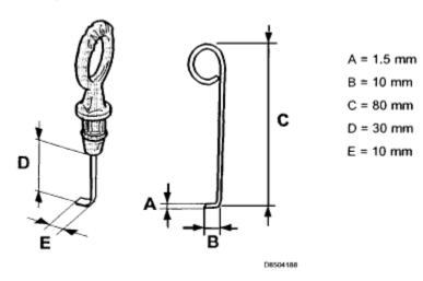
Make a tool from a welding rod, dip stick or similar. See the dimensions in the illustration.
