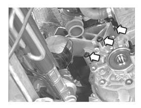
applied) under the left-hand side of the sub-frame. Remove the subframe screws. Lower the sub-frame.
