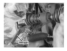
detach the drive shafts from the wheel hubs so that the gaiters are not damaged. Hold the spring struts away using a retaining strap to obtain better space when the drive shafts are removed.
