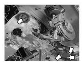
Installing the lefthand drive shaft to the gearbox and the wheel spindle
