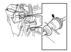
Check that the clip is positioned in the groove as illustrated.
