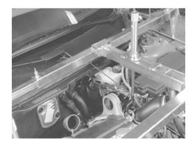
Fit the screws,  $7 \times M10$ , to the gearbox/engine.
