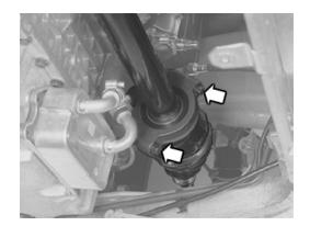
support bearing, 2 x M8. Tighten.
