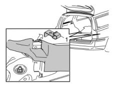
Remove the two mountings (1) for the front floor hatch on the right and left hand sides. The front floor hatch will not to be used again.
