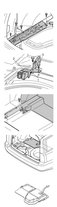
panel for the tail gate sill. If the car is equipped with a CD or RTI, reinstall the three screws for the CD bracket.
