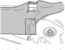
Tear off a small piece of the carpet following the existing perforations on the right and left-hand sides beside the shock absorber mountings.
