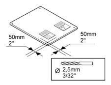
the four holes for pre-drilling as illustrated
