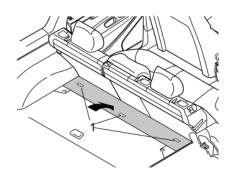
Press the front floor panel (from the kit) into the three clips (1).
