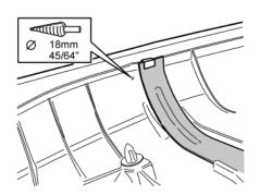
reinforcing rail on the inside of the panel
