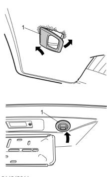
■ Take the tailgate opener panel (1) from the kit. Hook the panel on the inner panel on the tailgate opener. Press into place as illustrated.
