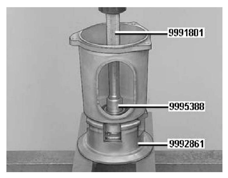
Support the viscous coupling housing on tool 999 2861. Press out the flange. Use drift 999 5388 with shaft 999 1801 or a suitable drift.
