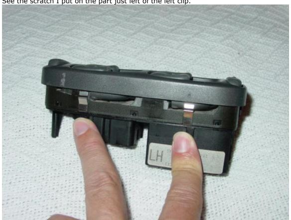
**2. Removing the Wire Clips**There are three wire bundle clips (gang clips) connected to the bottom of the master window controller.
