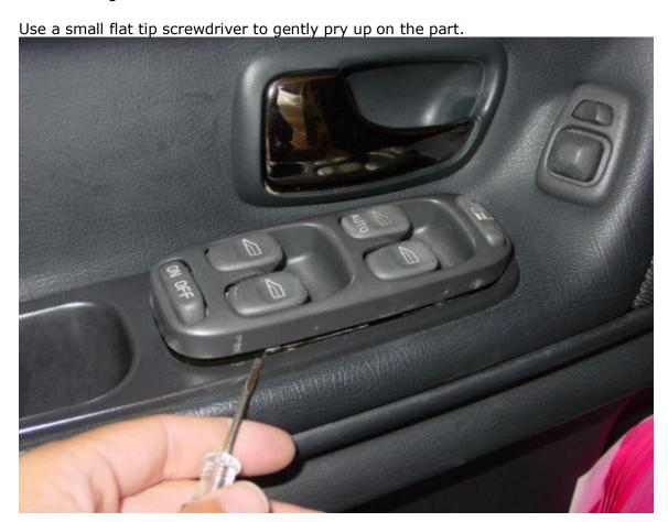
The part is held in place by four metal pressure/friction clips, two on each side. The clips are exactly 1-1/2 inches from each end. So when prying, try to be in this general area to get the best results. If you are going to reinstall the same part don't worry too much if you scratch the part while removing it because most scratches will be hidden by the door.
