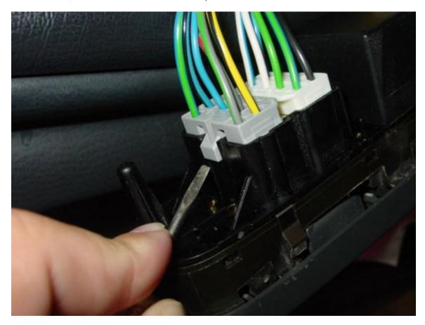
At first I had difficulty removing the clip. Then I pushed down on the wire clip and at the same time pushing in on the button/lever and then pulled up on the clip and it released. I did the same for the other two clips and had no problem.
