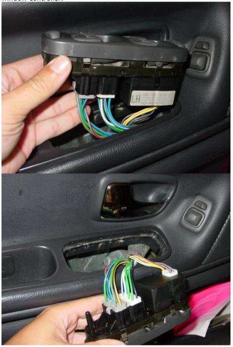
Never try to remove the clips by pulling on the wires. On the side of the clip is a small button/lever used to release the clip.
