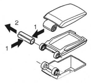
Pres the shaft together (1) and pull straight out (2). Separate the armrest
