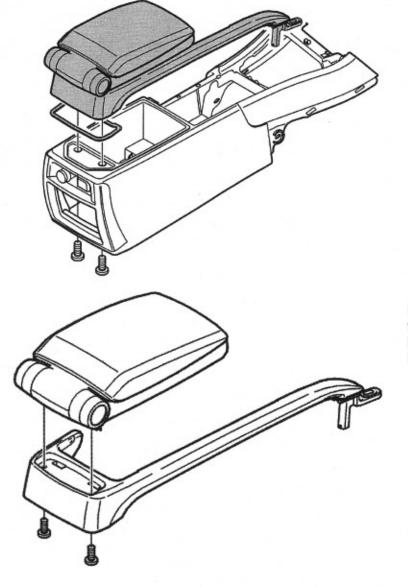
Remove the two screws from the rear edge. Remove the center console locker.
