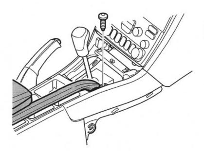
Remove the two screws. Press off the handle at the front edge of the center console.
