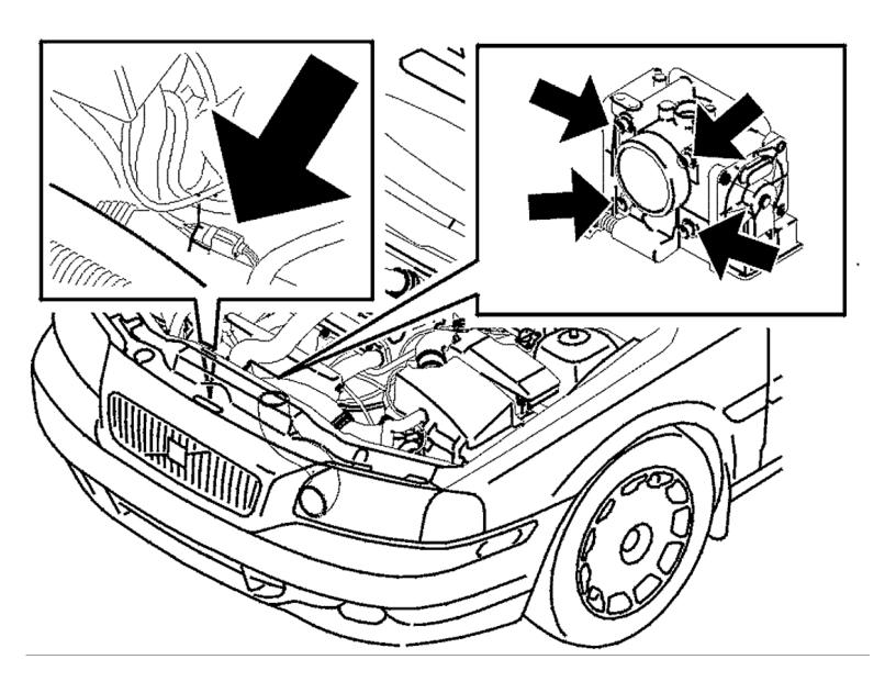
Disconnect the hose between the charge air cooler (CAC) and the throttle body (TB) at the end of the throttle body (TB). Move to one side.
