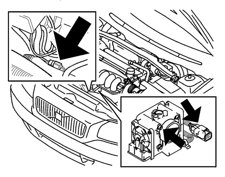
Disconnect the throttle body (TB) connector.
