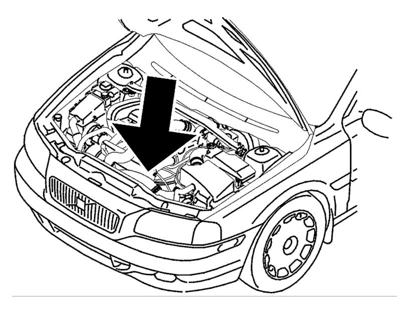
Remove the intake manifold between the front cover plate and the air cleaner (ACL) housing. Disconnect the battery negative lead.
