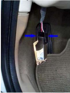
You will now be able to completely remove the lower panel from the carby pulling down and rearward on the panel.
