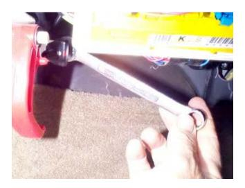
Turn the wrench in a clockwise direction (as you face the nut), or in a downward direction. This will extend the distance of the cable housing and remove the slack from the wire inside the cable housing.
