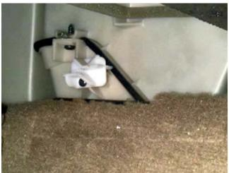
You will also need to keep the top of the panel low, towards the floor when you push the edges of the lower panel into the slides. Now push the courtesy light through from the bottom of the panel until it snaps in place and push the wire on until it clicks and locks. Lift the front of the panel upward, line up the two tabs in the panel with the slits in the upeer panel and push inward. Then simply reinstall the #25 Torx screw and you are done.
