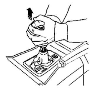
Stand astride the center console. Grasp the gear selector lever knob with both hands. Pull it straight upwards with a hard jerk.
