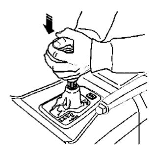
Press the gear selector knob so that it locks in the lever.
