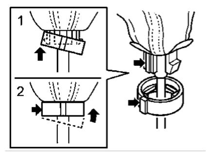
**Note:** The locking sleeve cut-out must be forwards so that it passes into the gear selector knob guide.
