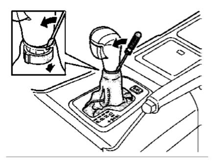
Insert a small screwdriver between the boot and the gear selector lever knob to access the lock bracket.
