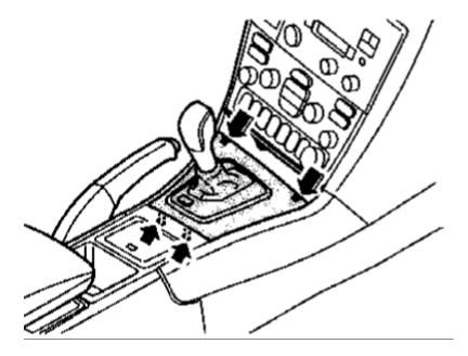
Angle the panel downwards. Press the top panel into place in the center console.
