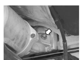
Filling and checking the oil in the final drive
