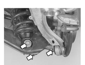
Installing shock absorbers, torque rods and anti-roll bar links (both sides)
