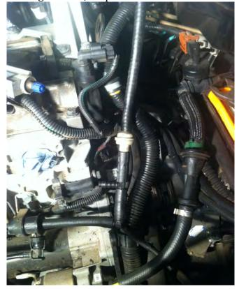
Installation is the reverse of this procedure. If you had to remove the thermostat housing, be sure to place the manifold gasket and the lower left bolt prior to reinstalling. Do a double and triple check to make sure everything that will be covered by the intake manifold is connected and routed properly. Take before and after pictures if it will help you remember.
