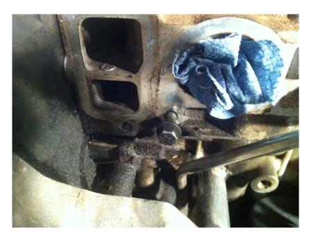
While I had the manifold gasket off, I replaced some brittle vacuum lines as well.
