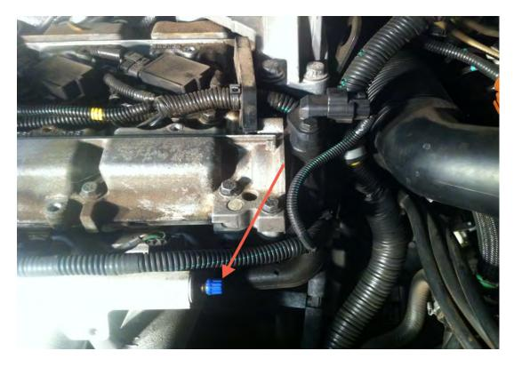
Remove the fuel rail mounting screws
