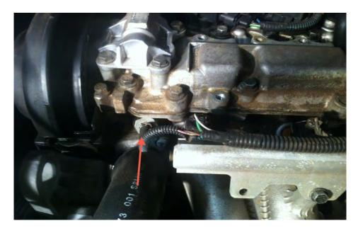
Spray a small amount of universal oil around the injector nozzles, then gently work the fuel rail up and down to loosen the injectors from their seat. You may have to perform the next step in conjunction with this step to remove the fuel rail.
