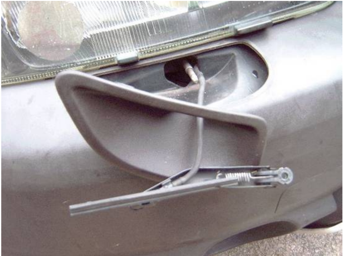
Wiper arm and removed filler plate (note pipe joint next to motor shaft)
