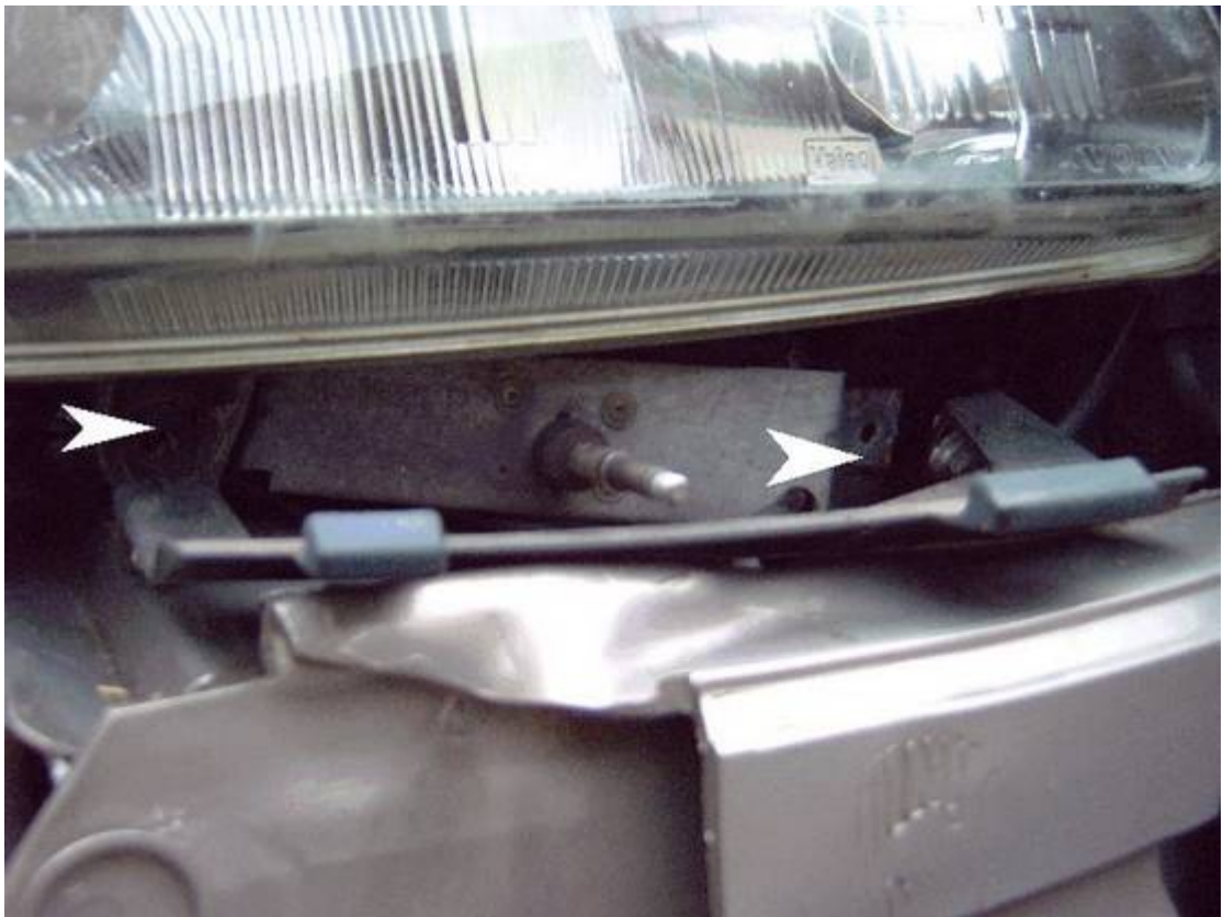
Wiper Motor fixing bolts (after they have been unscrewed)
