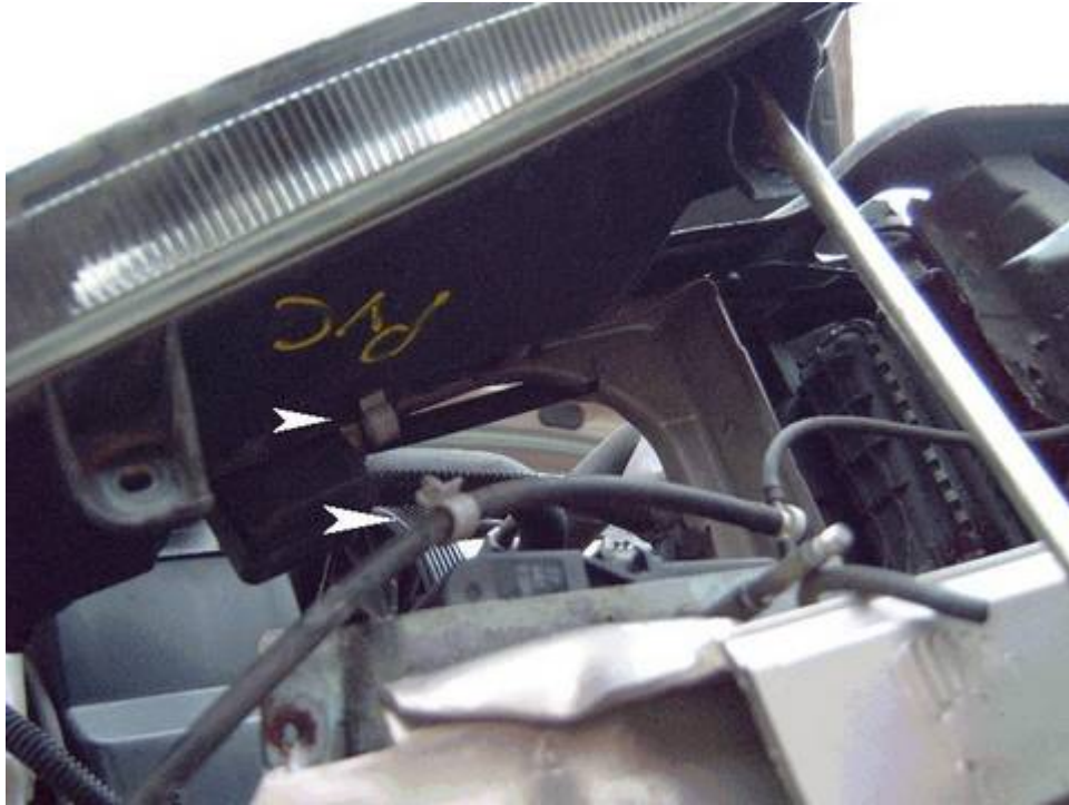
Underside headlight, clip shown on washer pipe, and also where fitted on replacement
