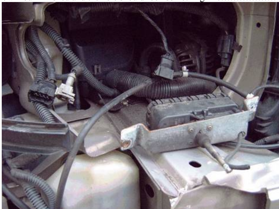
Underside headlight, clip shown on washer pipe, and also where fitted on replacement
