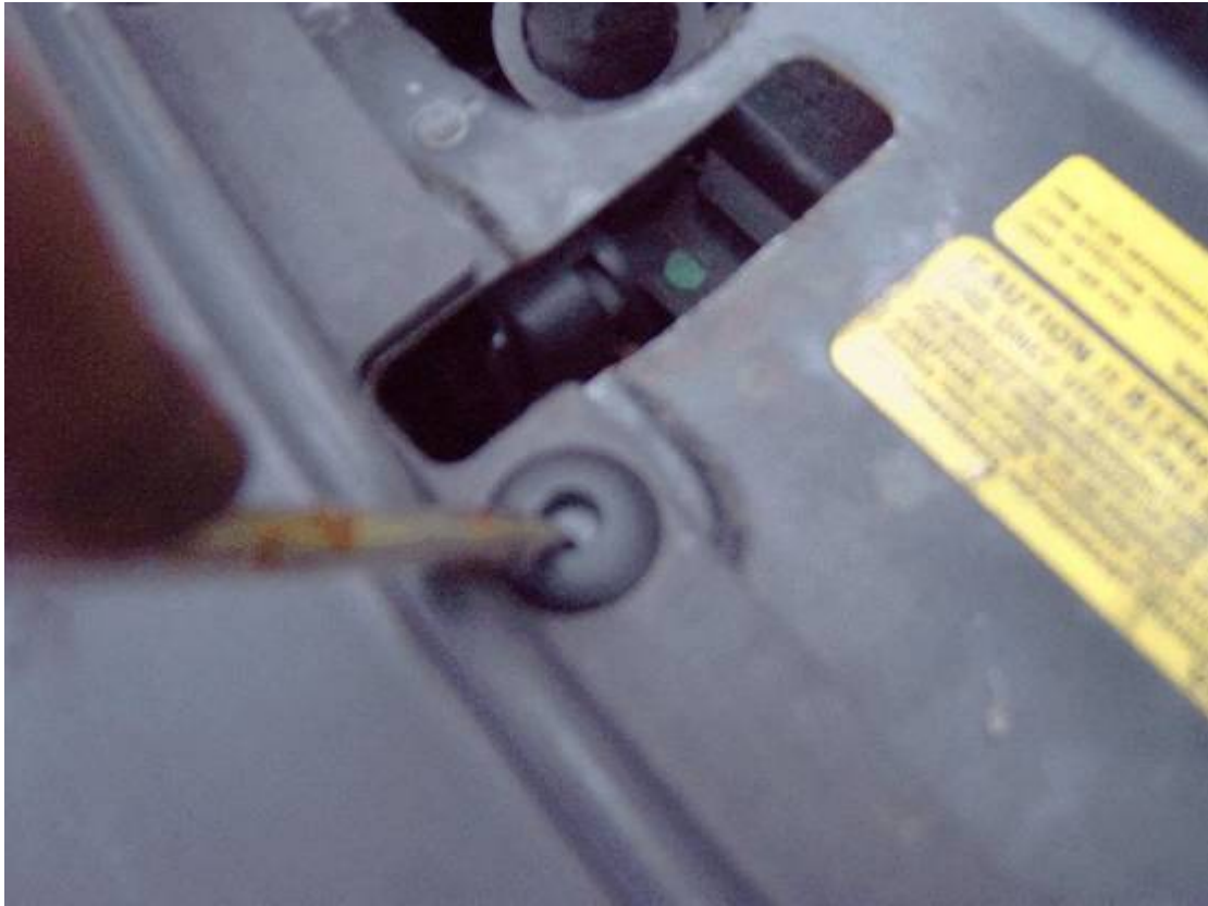
Releasing the push dot fixings
